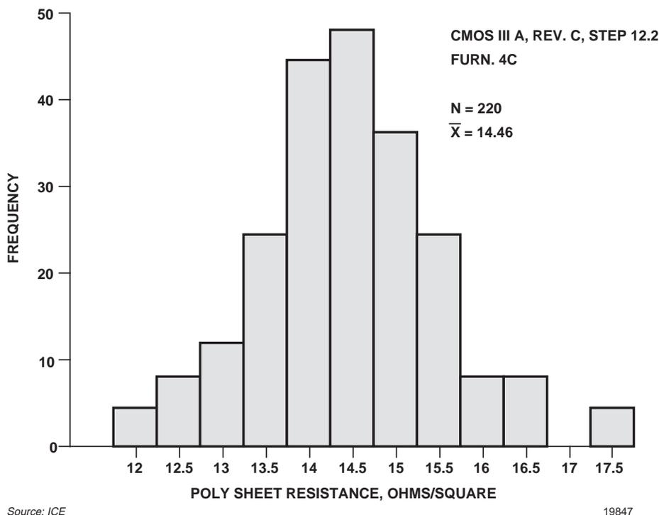
Figure 3-20. A Typical Histogram Shows the Distribution Around a Target Value
